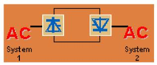
Fig. 4. Block diagram of back to back HVDC links.
