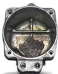
Abrasion compressor damage
