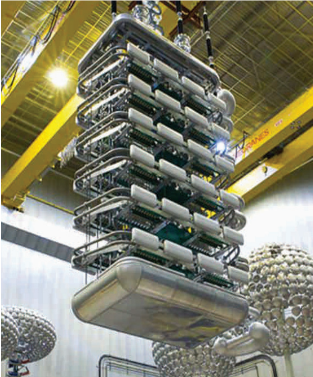
Thyristor Valves (for UHVDC application) under testing at STRI, Sweden
