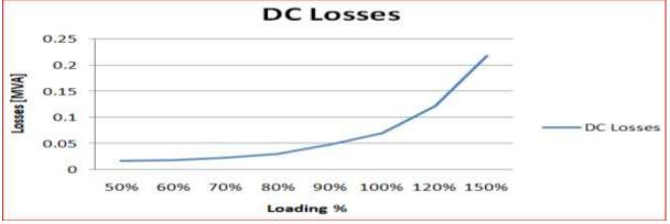
Figure 9: DC System Losses under different loading conditions
