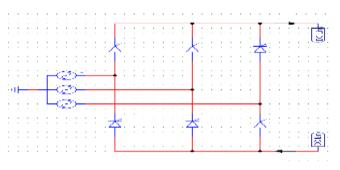
Figure:5 6- pulse LCC circuited. DC Cables
