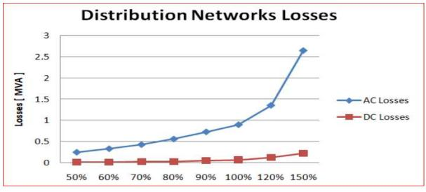
Figure 10 : AC & DC Systems Losses under different loading conditions.
